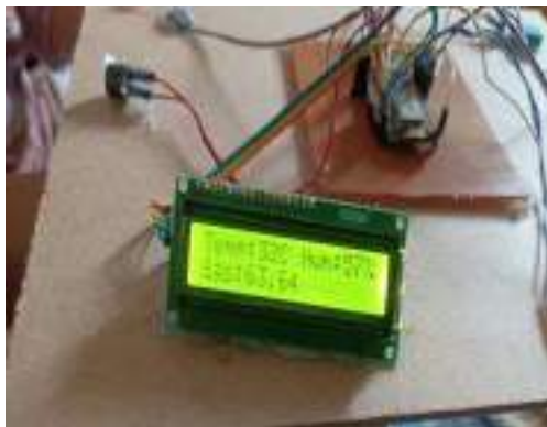
Figure5: Displaying the parameters measured on LED screen
