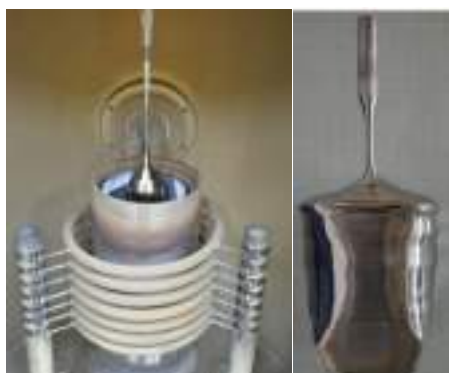
Germanium (Ge) single crystal (950 g) grown in CZ furnace
