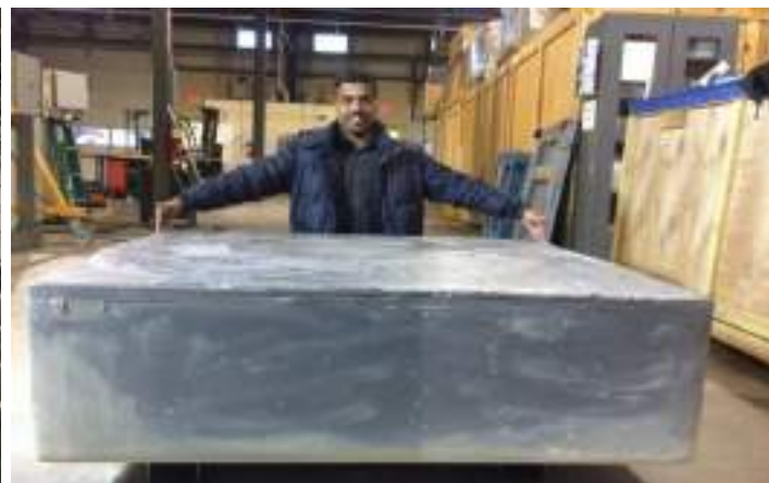
Multi-crystalline silicon grown by Dr. N. Balamurugan using Directional Solidification System (DSS) at China
