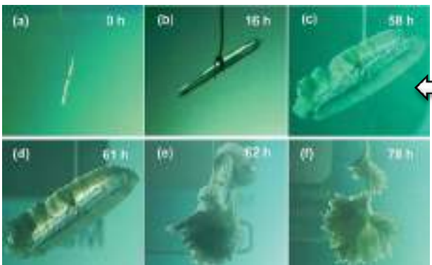
Growth progression of a vanillin single crystal in water without seed rotation by slow cooling: (a) the seed crystal, (b) growth of the seed with transparency and perfect morphology, (c) re-dissolution of the edges and oil entrapment in the center of the growing crystal, (d) terrace formation, (e) surface nucleation of leafy spike-like dendrites at the bottom and at the top, and (f) grown leafy spike-like dendrites at the end of the experiment
