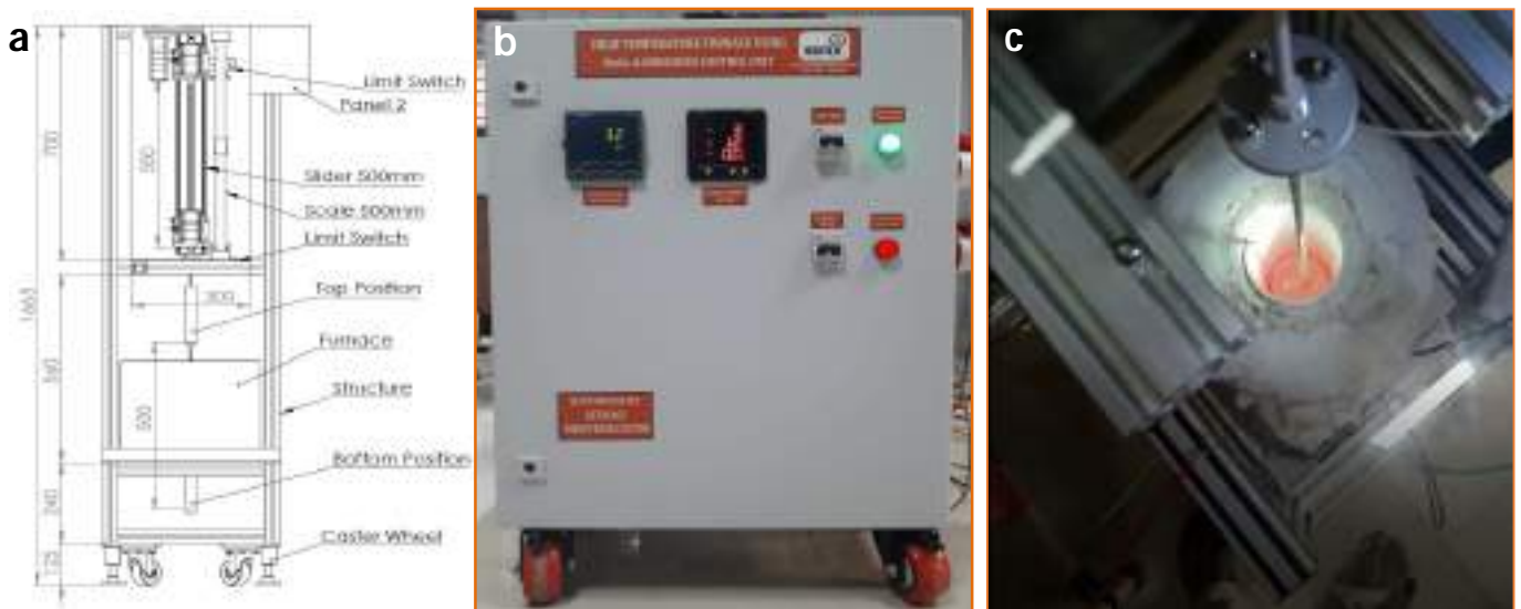
Figure.1 (a) Schematic Diagram of the Crystal Growth Puller, (b) High Temperature Furnace Control Unit, (c) High Temperature Furnace
