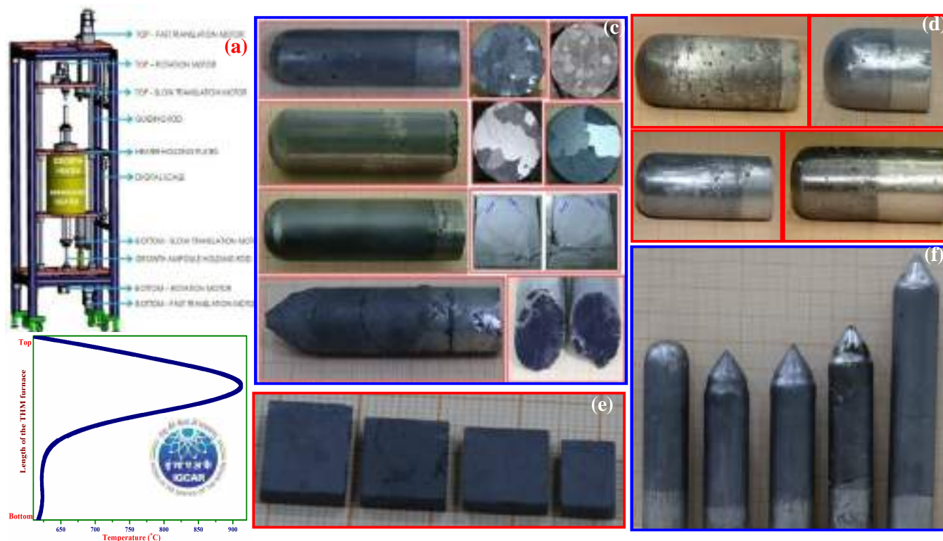
Figure.1 (a) Indigenously developed THM crystal growth system, (b) Temperature profile of two zone furnace, (c) Stages of CZT crystal growth (d) Optimization of CZT/Te ratio (e) CZT wafers and (f) As Grown CZT crystals (each growth run 60 days)
