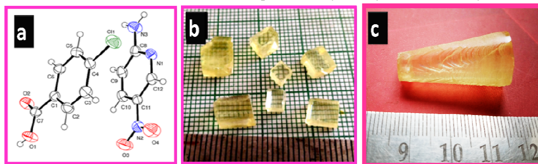
Figure. (a) ORTEP view of 2A5NP4CB with the atom numbering scheme, (b) SEST grown 2A5NP4CB single crystals and (c) SR method grown 2A5NP4CB single crystal
