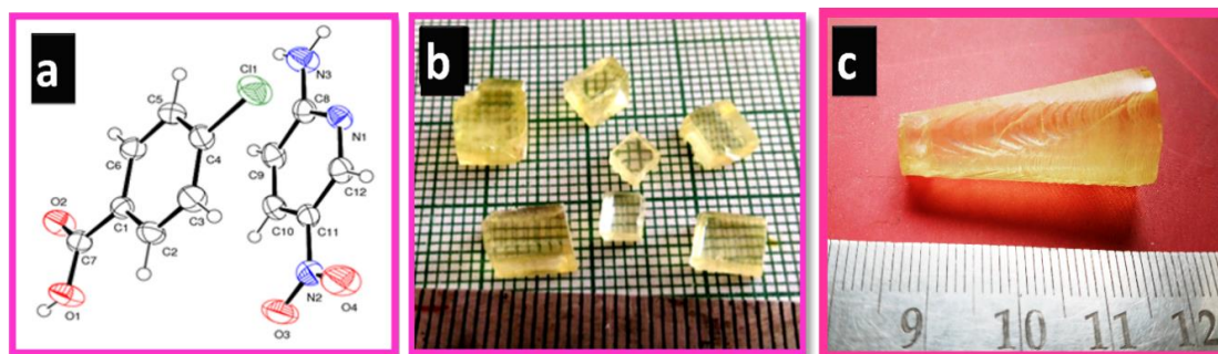
Figure 1. (a) ORTEP view of 2A5NP4CB with the atom numbering scheme, (b) SEST grown 2A5NP4CB single crystals and (c) SR method grown 2A5NP4CB single crystal
