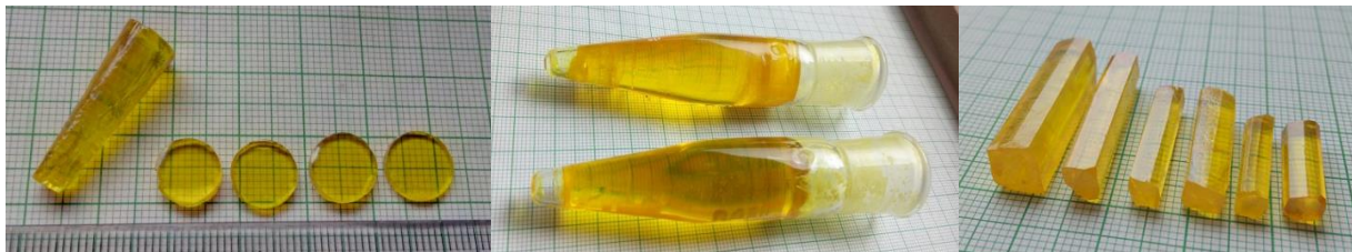
2AP4N crystals grown by (a) Conventional method, (b) SR method and (c) RSR method
