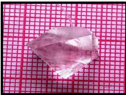
Figure: Photograph of as grown p-Toluidinium nitrate crystal
