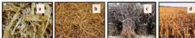
Figure 1: Potential non-wood fibre sources for paper making (a. bagasse, b. wheat straw, c. cotton stalks, d. corn stalks)
