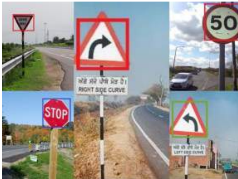
Figure 4 Examples of some road sign detection by the proposed algorithm on the Indian road signs
