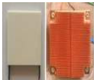
Thermo electric generator
