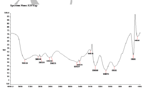
Fig .2a FT-IR spectra of 5 mole thiourea doped KDP crystal
