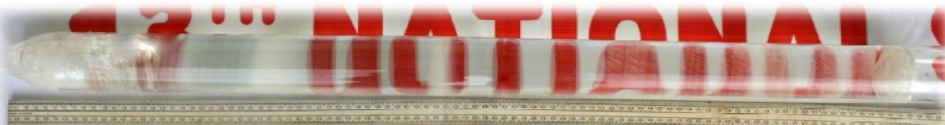
1350 mm long unidirectional method grown crystal – 2012 - M.Senthil Pandian and K. Boopathi
