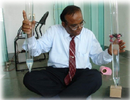
650 mm long unidirectional method grown crystal – 2008 M. Arivanandhan et. al.
