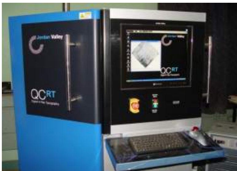
Fig 1. X-ray topography system for defects characterization of single crystals at RRCAT, Indore
