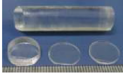
Above T c grown TGS crystal Dr.Muthu Senthil Pandian et. al. SSNCE
