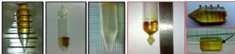
Photos of 8-HQ single crystal growth from VBT (a) during growth (b) crystal with ampoule (c) harvested crystal
