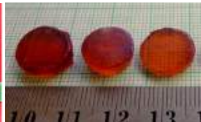
LAPP crystal grown by SR method Dr.Muthu Senthil Pandian et. al. SSN RC
