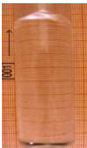
Fig 1. Unidirectional grown DKDP crystal, dia. 19mm, length 81 mm
