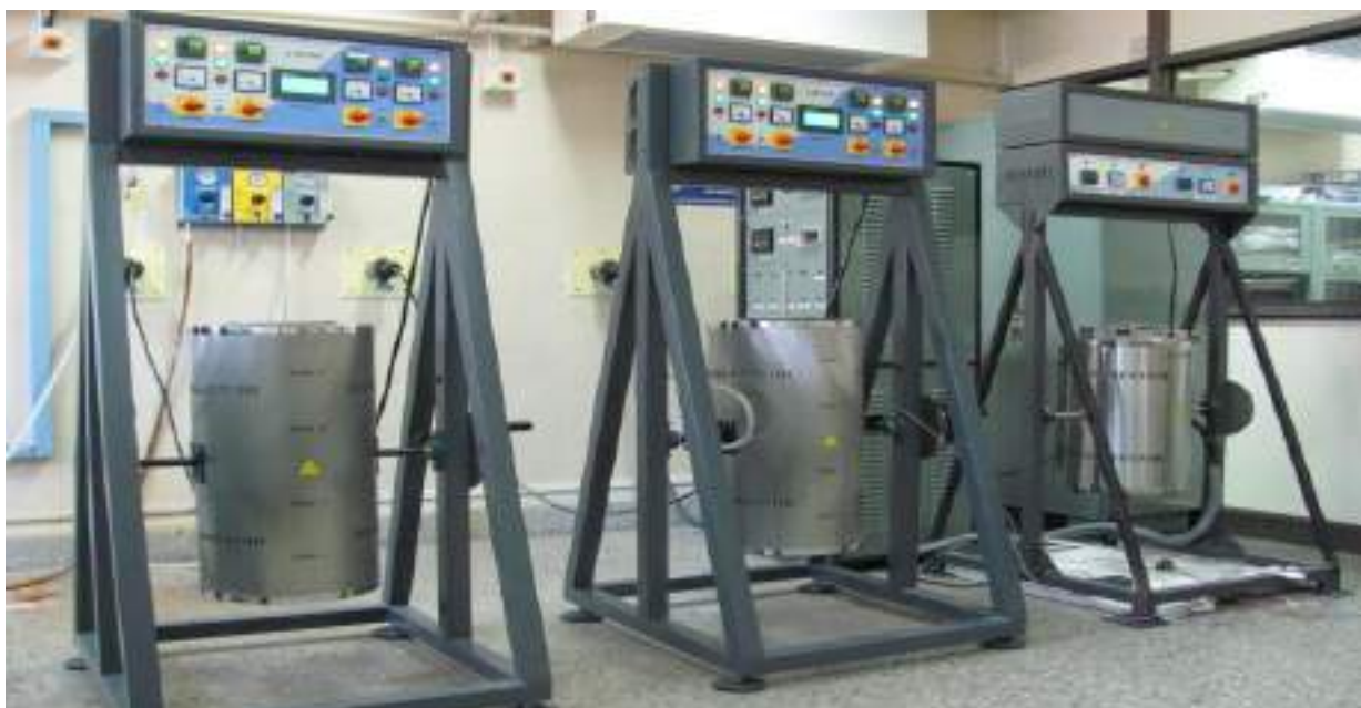
Fig 1. Modified Bridgman systems developed for industrial production of CsI:Tl and NaI:Tl scintillator crystals
