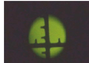
A device based on GGAG:Ce crystal and a CCD to record spatial profiles of X-ray beam. The photograph shows the image of an X-ray beam having 2 mm diameter
