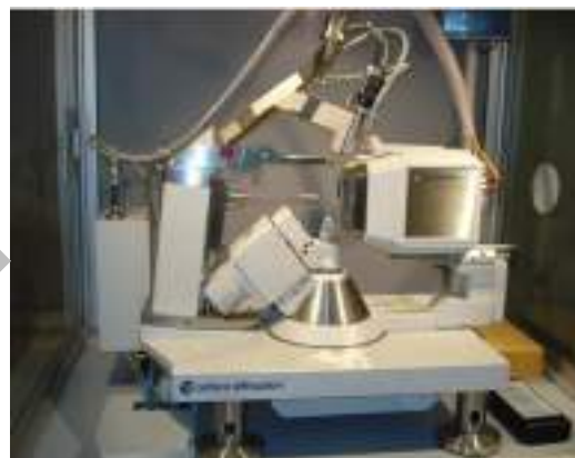
Goniometer Set-up for the DST- XRD National Facility
