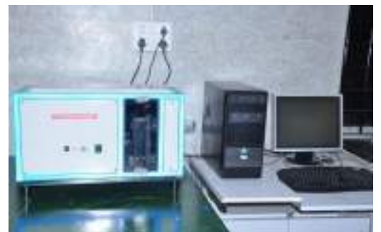
Fig.2 The photograph of the fabricated Photoacoustic spectrometer
