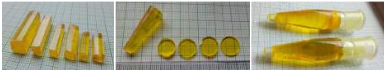
2AP4N grown by (a) Conventional method, (b) SR method and (c) RSR method
