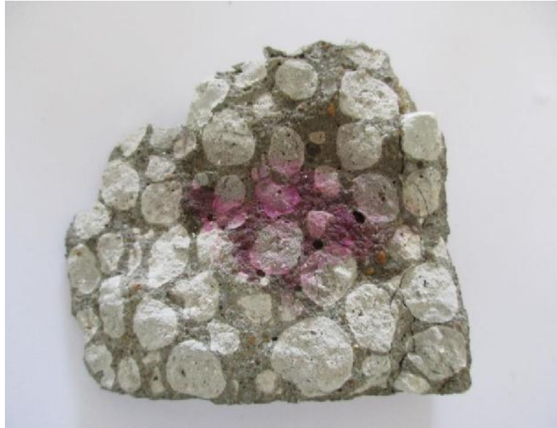
Fig 9a. Pink colour indicates the basic pH of (WAP) concrete
