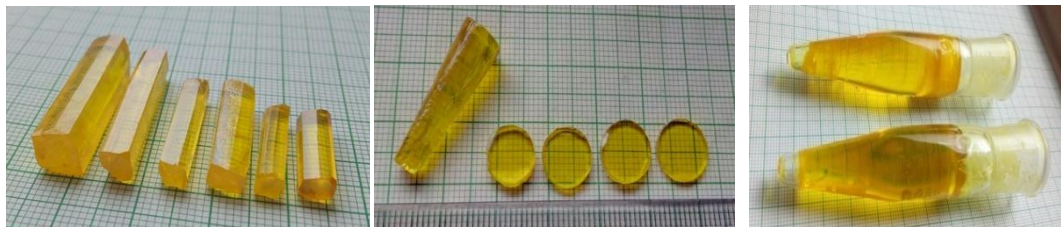
2AP4N crystals grown by (a) Conventional method, (b) SR method and (c) RSR method
